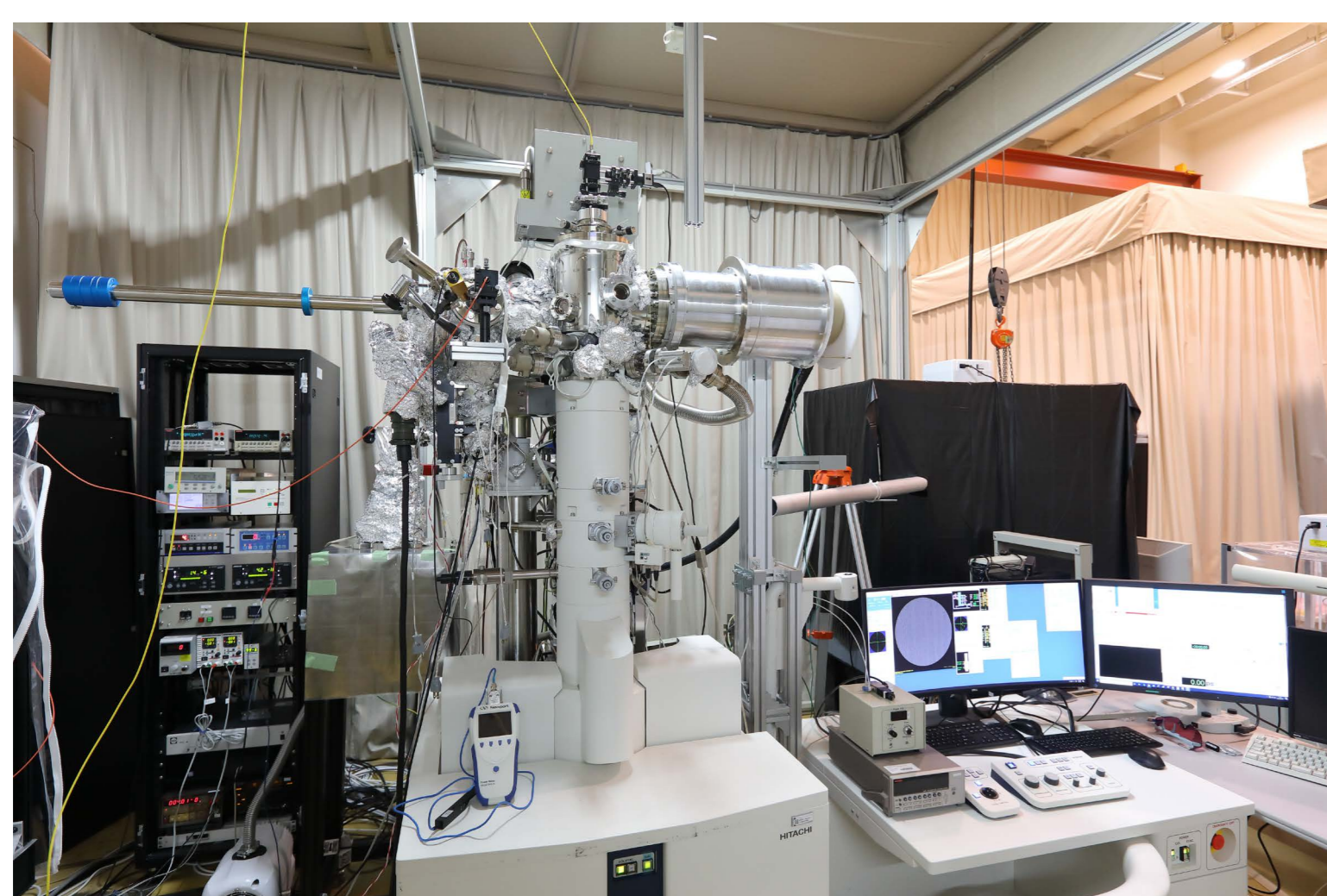
A semiconductor with an NEA surface is equipped in the photocathode-type e-gun. The extra-high vacuum and high acceleration field in the electron gun was realized simultaneously.
