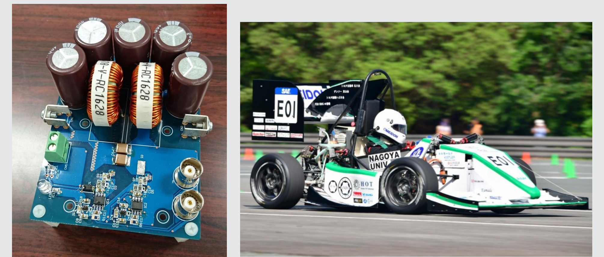
Inverter circuit board with gallium nitride (Left Side), Nagoya University Student Formula FEM (Right Side)
