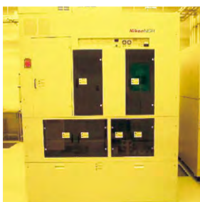
i線ステッパ Nikon NSR-2205i12D i-line stepper Nikon NSR-2205i12D
