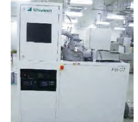
ALD(プラズマ式/サーマル式) Ultratech/CambridgeNanoTech Fiji G2 Atomic layer deposition system (Plasma/Thermal) Ultratech/CambridgeNanoTech Fiji G2
