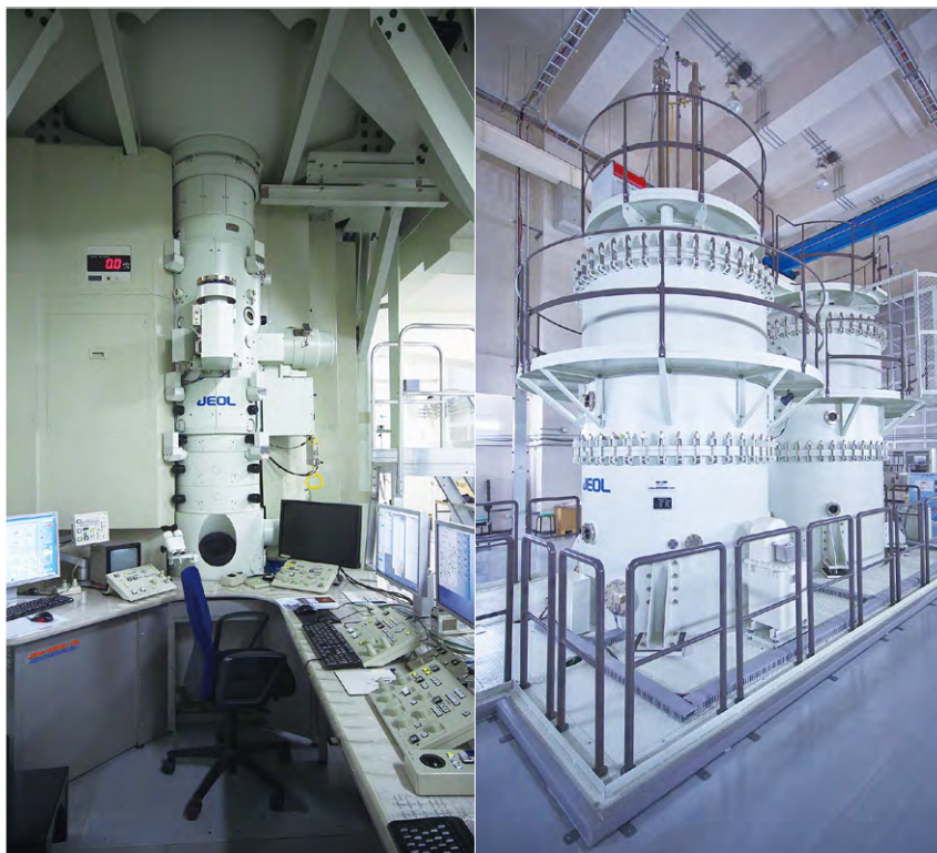
反応科学超高压走査透過電子顕微鏡 JEM1000K RS Reaction science high voltage scanning transmission electron microscope (JEM 1000K RS)
