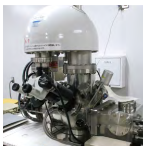
X線光電子分光装置 ESCA-3300 X-ray photoelectron spectrometer ESCA-3300
