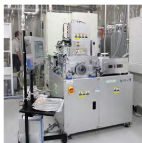
高温スパッタ成膜装置 ULVAC QAM4 High Temperature Sputtering Deposition Equipment ULVAC QAM4
