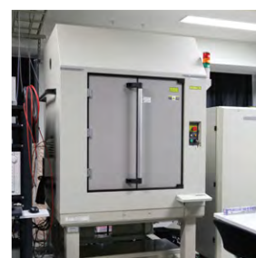
エミッション顕微鏡 HAMAMATSU PHOTONICS PHEMOS-1000 Emission microscope HAMAMATSU PHOTONICS PHEMOS-1000
