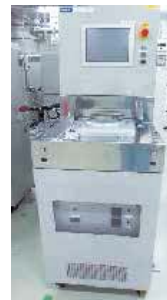
P-CVD1 samco PD-220NL Plasma CVD 1 samco PD-220NL
