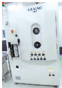
EB蒸着装置 ULVAC ei-5 EB evaporator ULVAC ei-5
