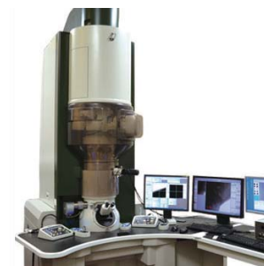
電界放出型走査透過電子顕微鏡 JEM-10000BU (収差補正電子顕微鏡) Aberration corrected scanning TEM JEM-10000BU
