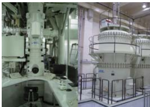
反応科学超高圧走査透過電子顕微鏡 JEM1000K RS Reaction science high voltage scanning transmission electron microscope (JEM 1000K RS)
