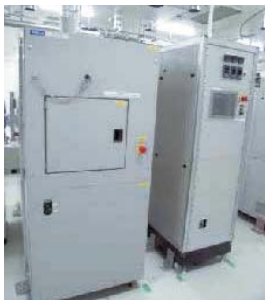
LP-CVD samco LPD-1200 Low pressure CVD system samco LPD-1200
