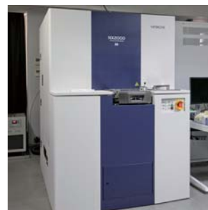
FIB-SEM HITACHI NX2000 FIB-SEM HITACHI NX2000
